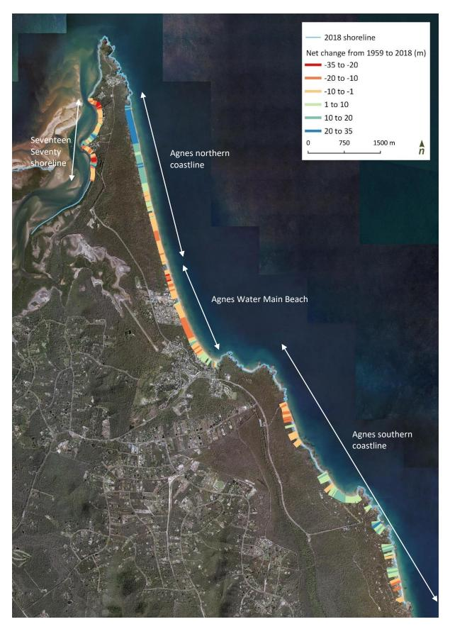
**Figure 19.** Net shoreline movement from 1959 to 2018 (m) – seaward accretion (+ve change) or landward recession (-ve change) measured from transects spaced at 20 m intervals along the shoreline
