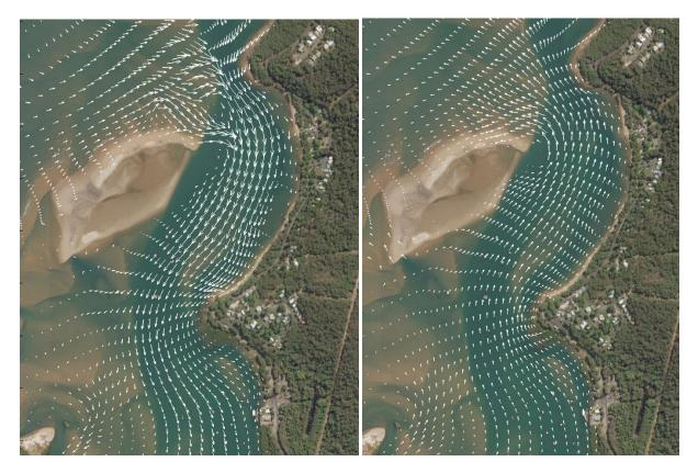
Figure 8. Modelled tidal patterns during flood tide (left) and ebb tide (right)
